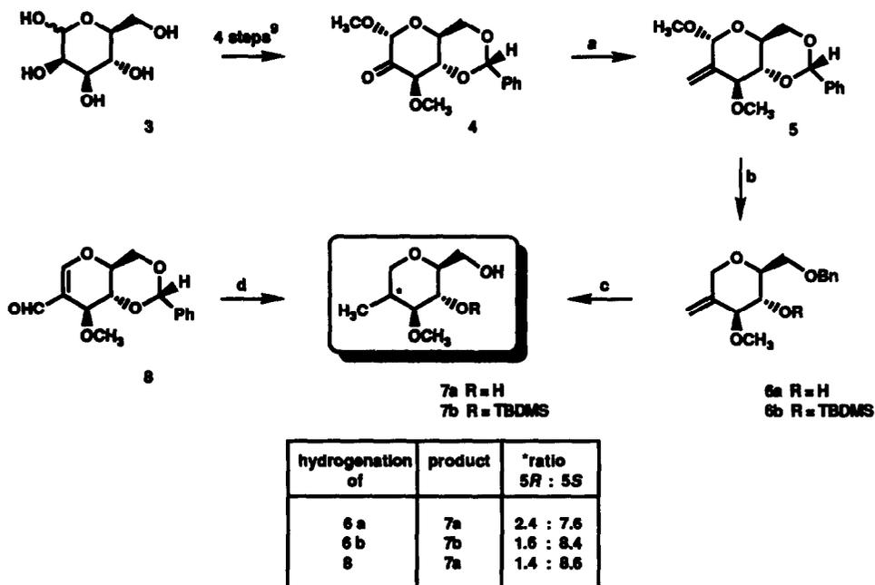
**Scheme 2.** (a) Ph<sub>3</sub>PCH<sub>3</sub>Cl, n-BuLi, THF, -20°C → r.t. (b) NaCNBH<sub>3</sub>, THF, slow addn. of ether/HCl<sub>gas</sub> (c) H<sub>2</sub>, Pd/C, EtOAc or THF, separation of isomers **7b** by MPLC on silica with pentane/EtOAc (d) H<sub>2</sub>, Pd/C, MeOH.
